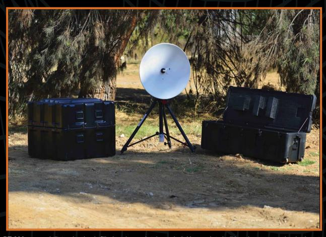
The OS-PT-200 pan and tilt tracker is air-filled and completely sealed. Heavy-duty ball bearings supporting both output shaft allow it to accommodate heavy antenna arrays. Each axis includes a DC brushless stepper motor coupled with zero backlash rigid worm. The unit has been designed to operate under harsh environment where rain, humidity, and dust are issues. It features continuous rotation of the pan axis and a self-locking mechanism, so when power loss occurs it stays in position.
